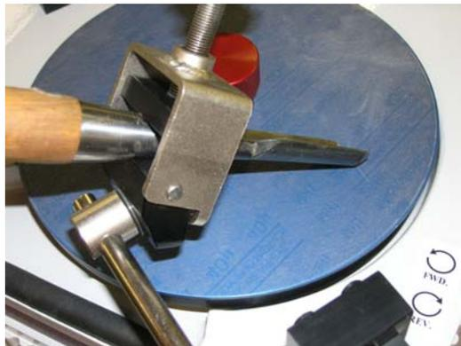
**Sharpening Large Gouge using Pivot Clamp**
